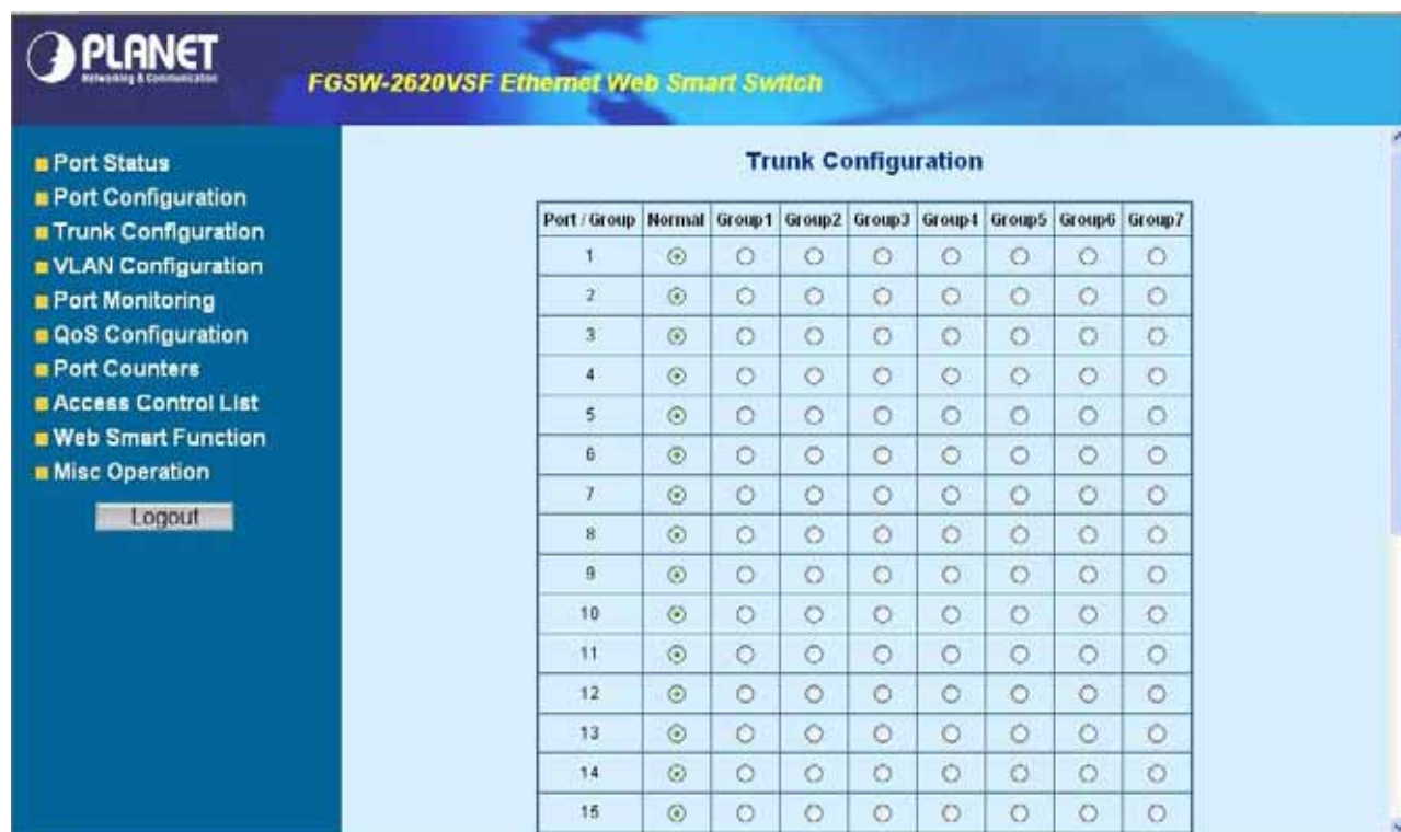
Figure 4-6 Trunk Configuration Web Page screen
